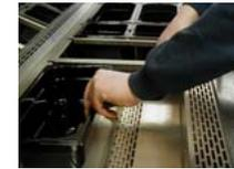
3. To clean the perforated ‘air return grill’, remove the perforated ‘air return grill’ using the finger holes provided as illustrated below. Use a warm soapy solution to clean.
